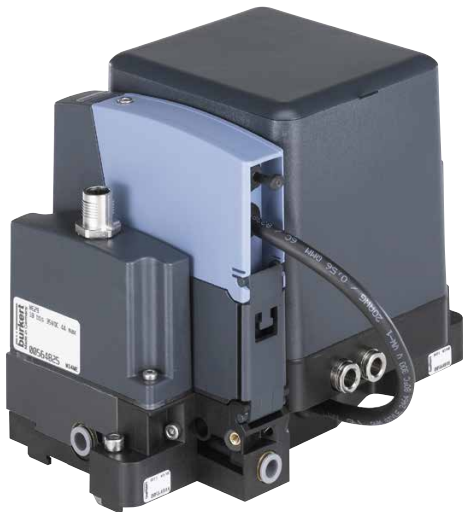
Automatic Cleaning System consisting of a cleaning module Type MZ20 directly connected to one Sensor Cube Type MSxx. On the left side is the I/O Module Type ME24 which provides the control of the cleaning module.
