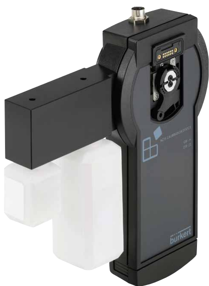
Handheld calibration unit Type MZ15: Calibration can be done by plugging in the right calibration buffer and the Sensor Cube. Operation is controlled via a connected Bürkert Communicator or a Type 8905 system with 7" touch display.
